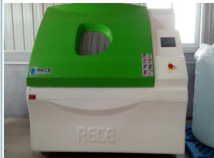
condensate water testing machine
